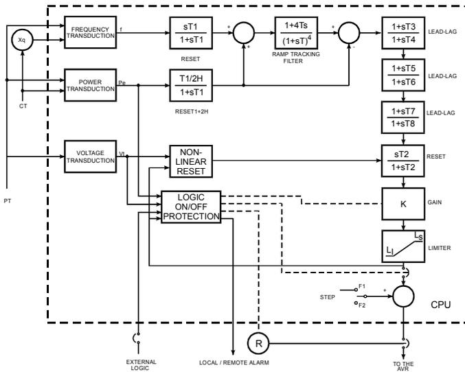
FIGURE 3 - PWX500 Block Diagram.
