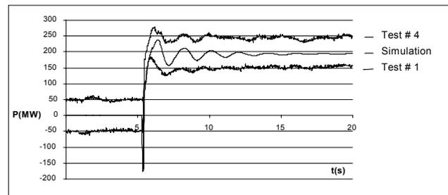
FIGURE 13 - Active power: El Chocón - Puelches line.
