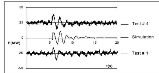
FIGURE 14- Active power: Rincón - Resistencia line.
