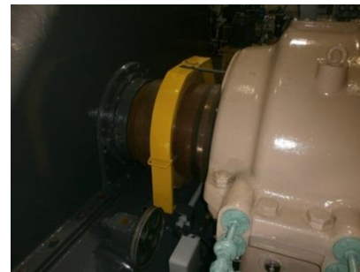
b) New system: Inductive sensor
